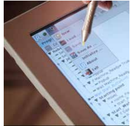
The CoWelder is easy to program by means of the robot arm and teach pendant with 12" touch screen.
