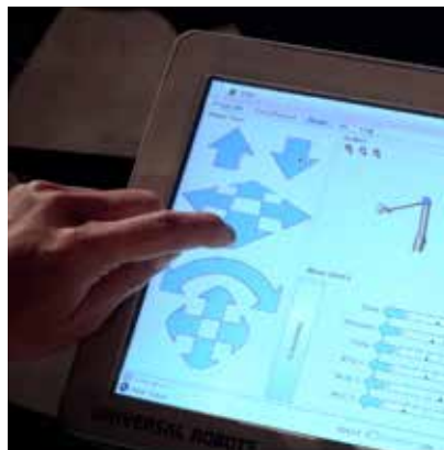
The CoWelder is easy to program by means of the robot arm and teach pendant with 12" touch screen.
